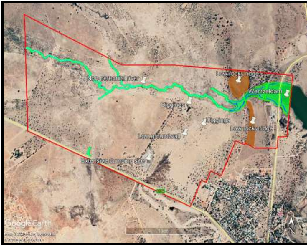
Figure 6. Indication of non-perennial river (active channel, riparian zone, buffer zone), in-channel dam and low rocky ridges at the site.
