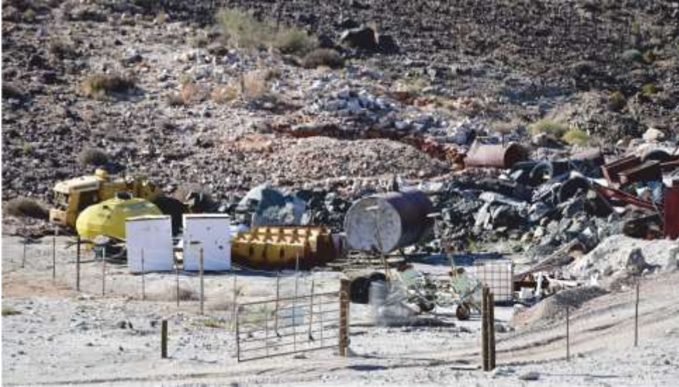
Photo 18: Recently fenced salvage yard. Note the large tank is currently used for used oil storage. This needs a bund, or can be replaced by the 1000L tanks (but must still be supplied with a bund).
