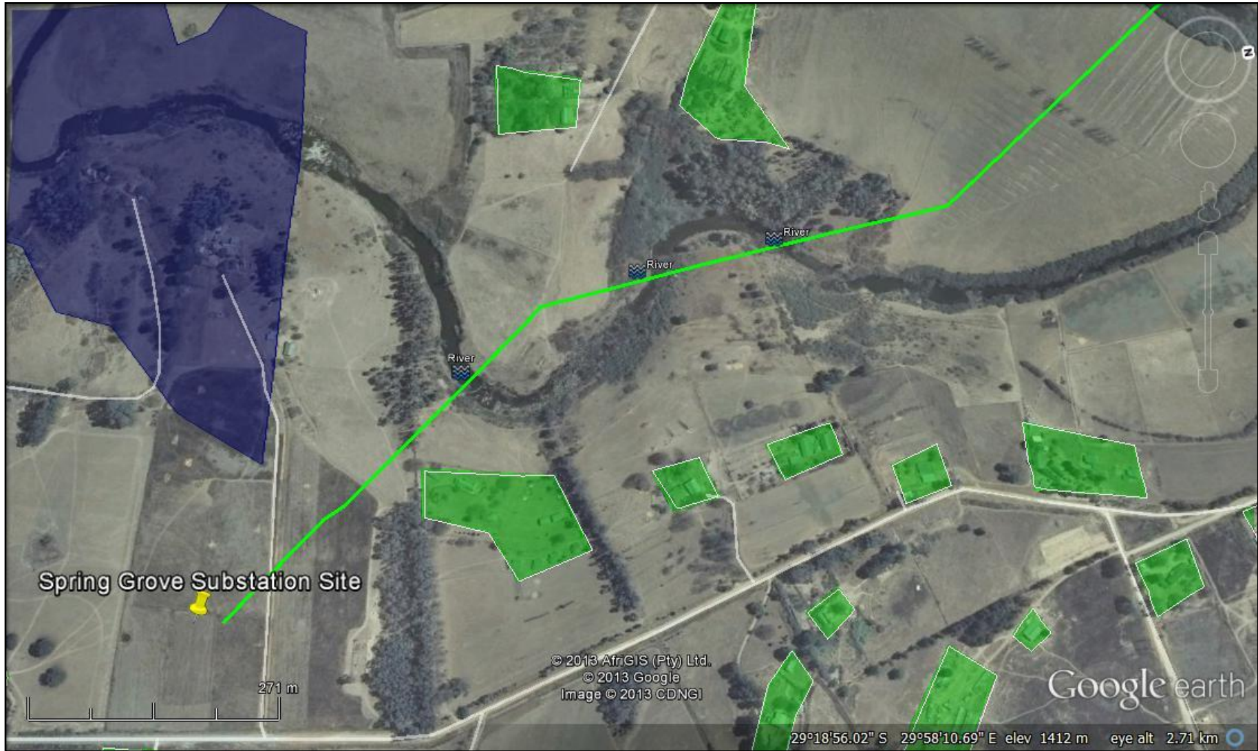
Figure 14: Close up aerial image of the Wetland/River/Stream/Drainage lines identified by the Wetland Specialists that the Alternative C3 Spring Grove Tee 88kV Powerline traverses (Source: Google Earth, 2013).
