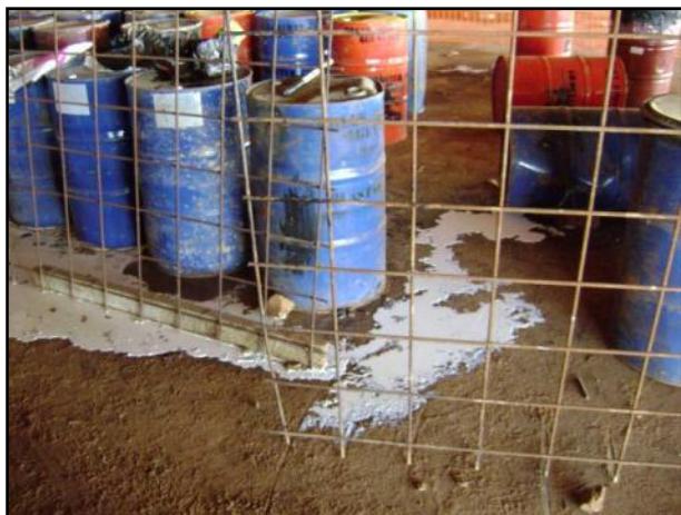
Figure 19: An example of hazardous material which has not been properly stored and is leaking on to bare soil. Hazardous material must always be kept separate from other storage areas and must be banded.
