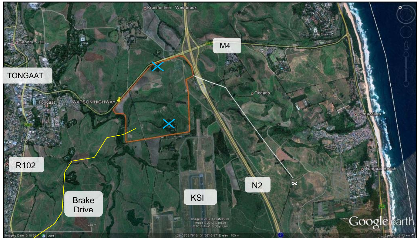
Figure 1: Aerial photograph of the location of the proposed uShukela Highway Development site (orange). The proposed water pipeline route is shown in white and the proposed water reservoir by the white cross. Blue crosses indicate the approximate positions of the two culturally significant structures older than 60 years (Source: Google Earth).
