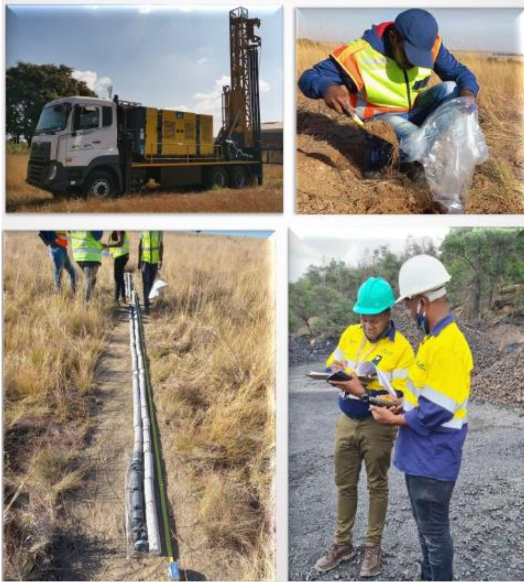
Figure 9: Geological Core logging and sampling
