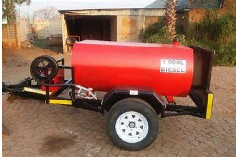
FIGURE 12: EXAMPLE OF AN ABOVE-GROUND DIESEL STORAGE TANKS.
