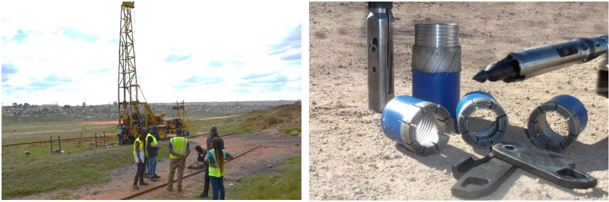
FIGURE 4: TYPICAL EXAMPLE OF DIAMOND CORE DRILL RIG AND DRILL BITS.
