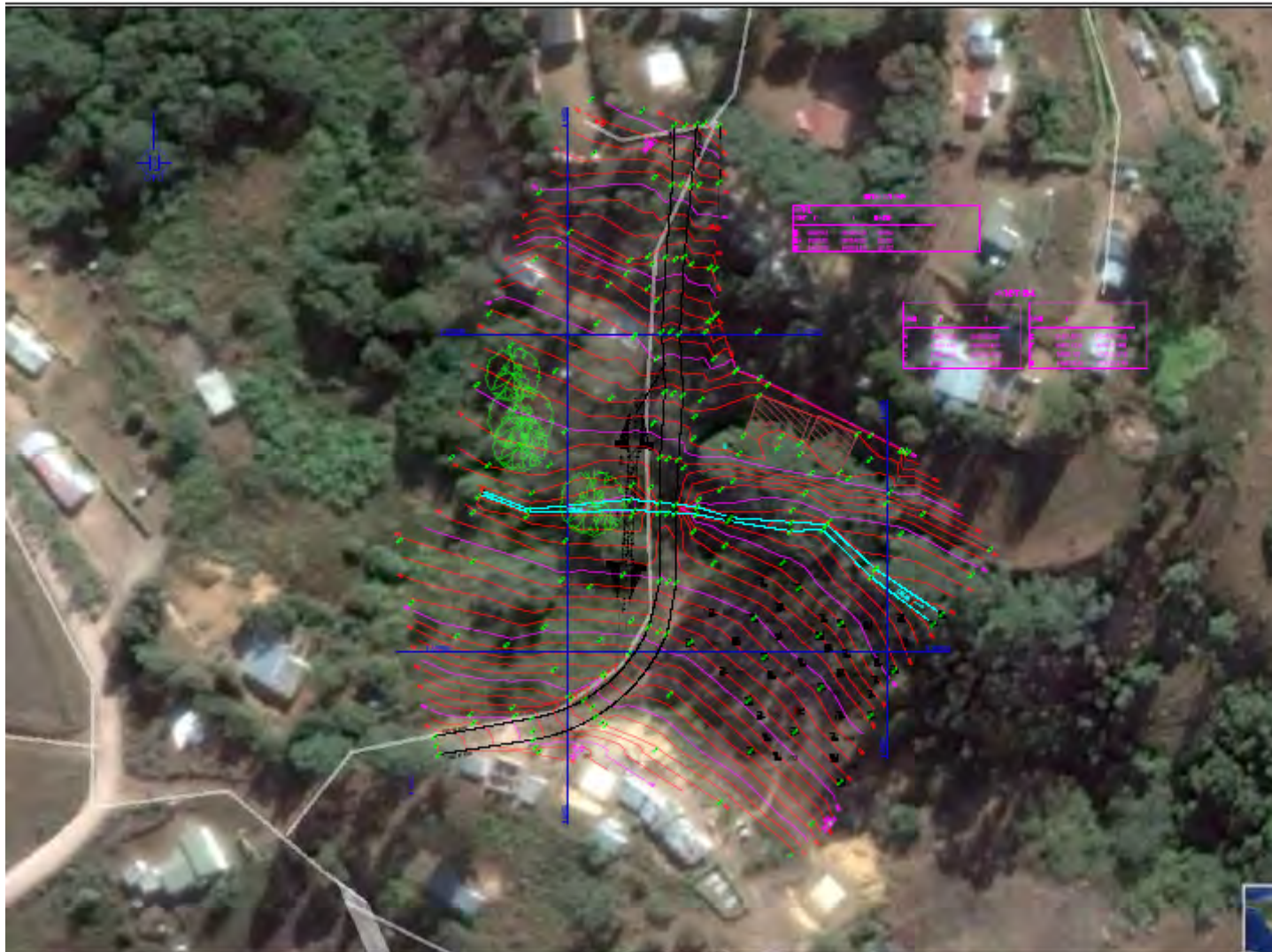
Figure 2: Proposed Layout of Dressing Bridge
