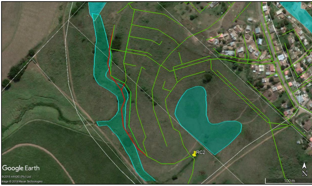
Figure 2: Red pipeline showing the original layout for the proposed sewer pipeline with the green lines showing the amended pipeline which has been re-located outside of the wetland area in the preferred layout.
