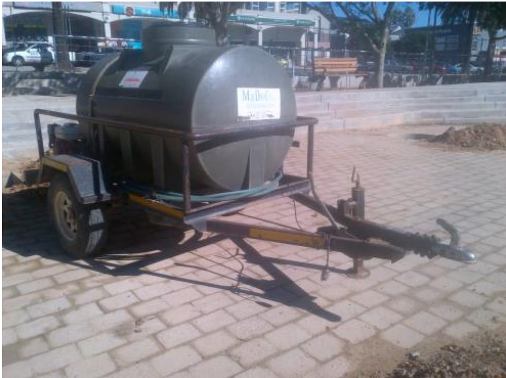
Figure: Indicating a mobile water cart
