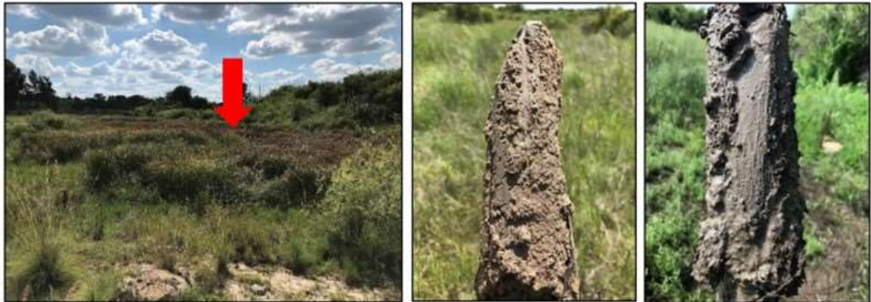
Figure 26: : A depiction of responsive (saturated) soils associated with the pan and valley bottom.
