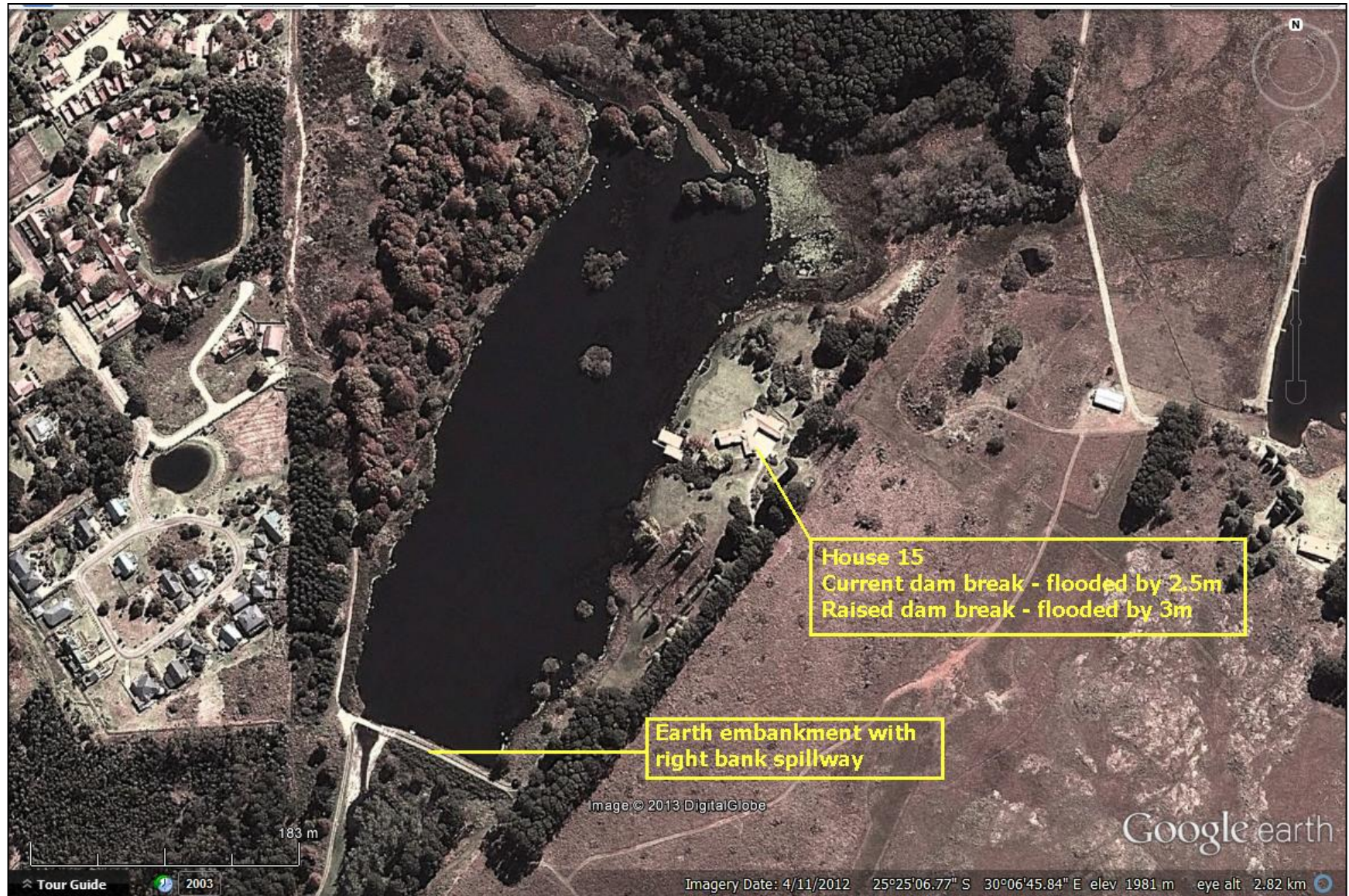
Figure 9-4 : Dam Break Assessment – Lower Reach
