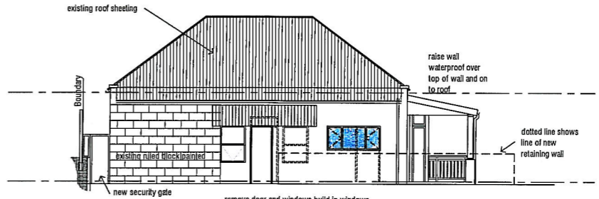
NORTH WEST ELEVATION
