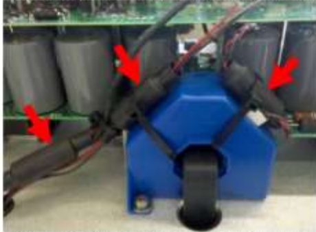
Analog Signal Conditioning using Ferrite Beads
