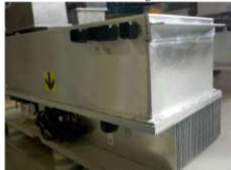
Power Electronics Enclosure for EMI Shielding
