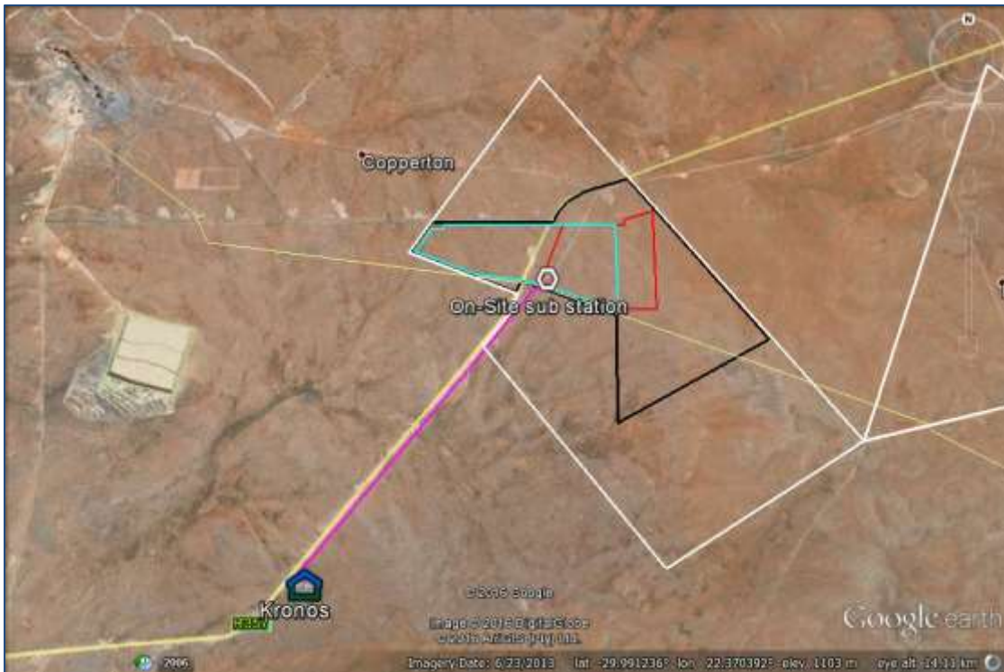
Figure 1: Satellite image of the Humansrus Solar 3 SEF illustrating the property boundaries (white), study area (black), preferred site layout (red), alternative site layout (blue), location of the on-site substation, and grid connection to the Kronos Eskom substation (purple).
