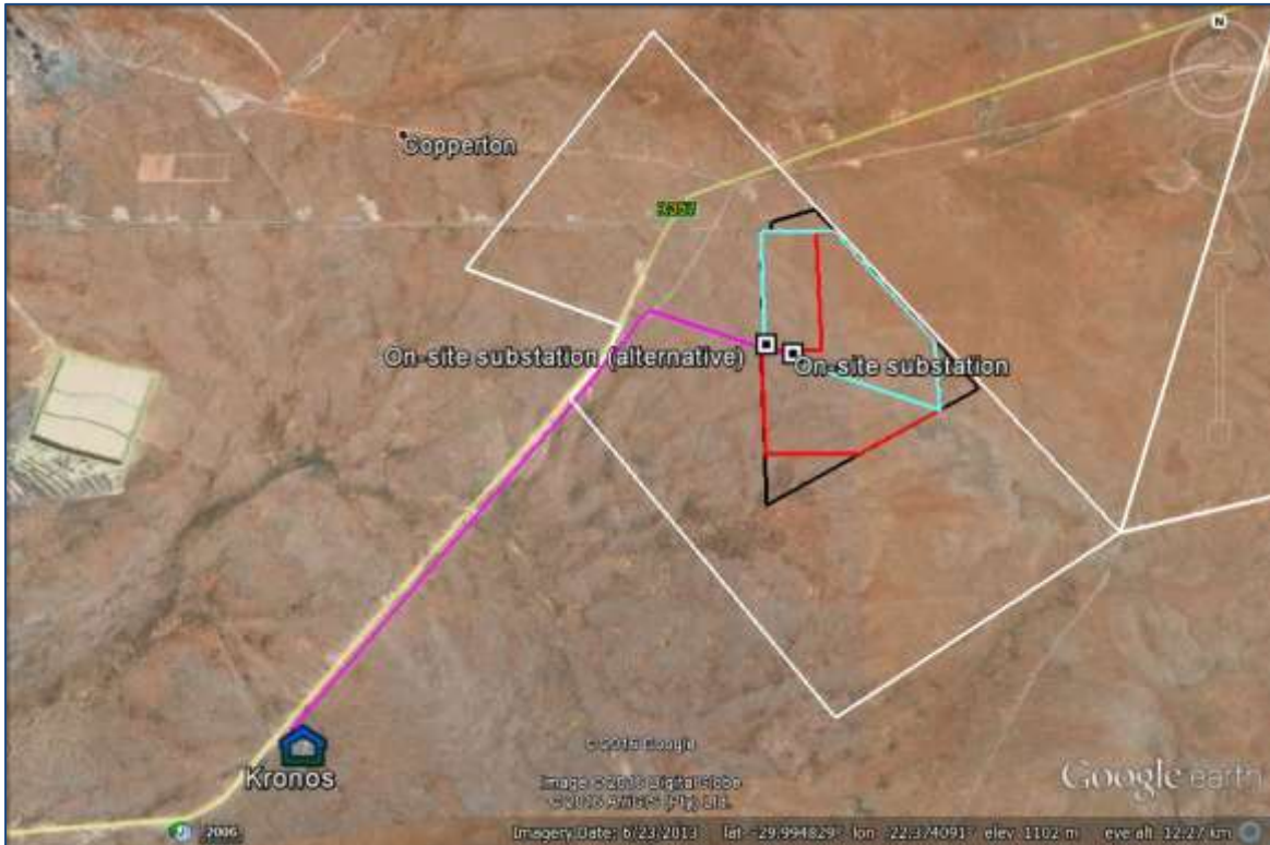
Figure 1: Satellite image of the Humansrus Solar 4 energy facility illustrating the property boundaries (white), study area (black), preferred site layout (red), alternative site layout (blue), location of the on-site substation, and grid connection to the Kronos Eskom substation (purple).
