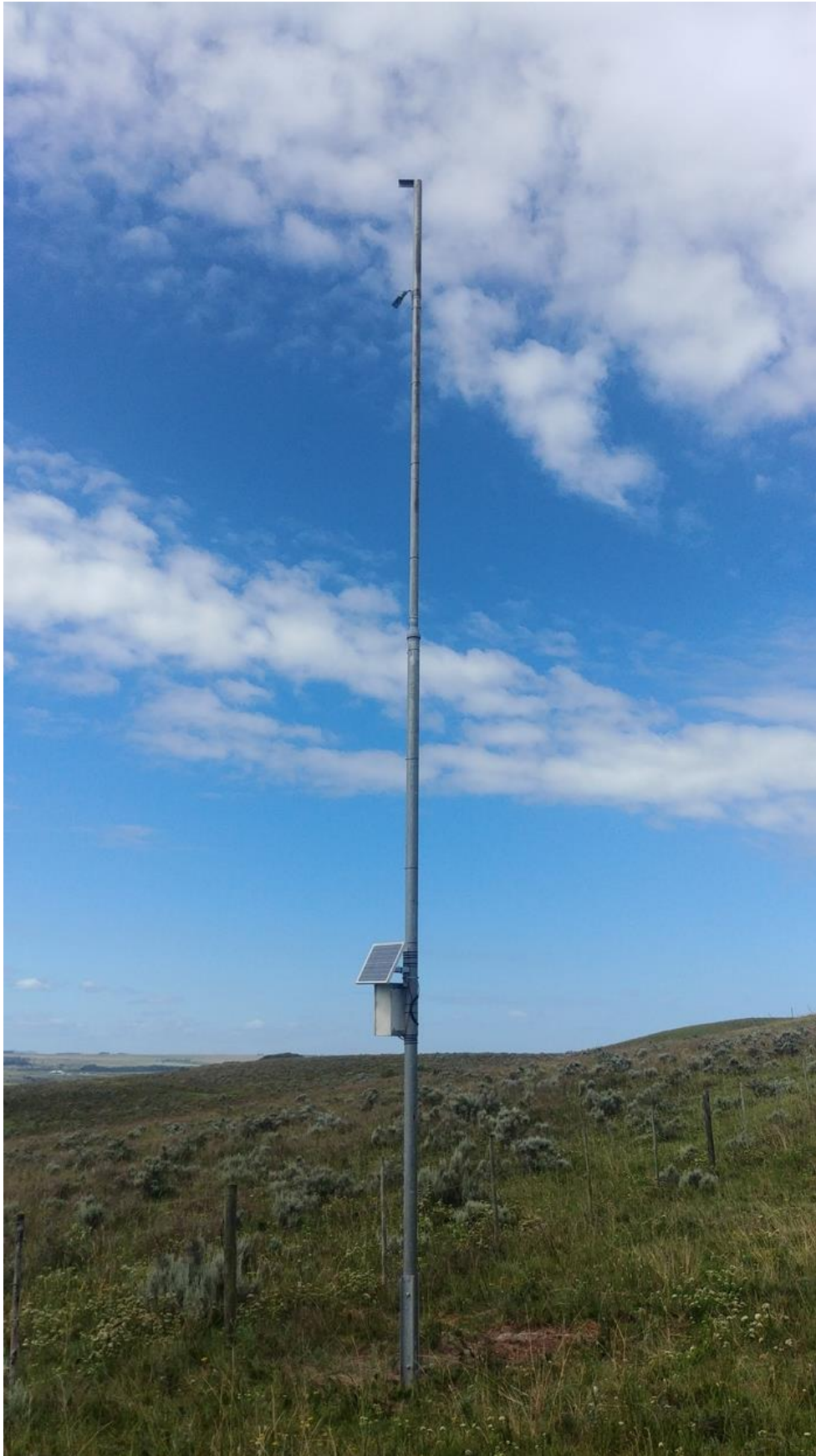
Figure 3.2: One of the Short Mast systems set up on site.
