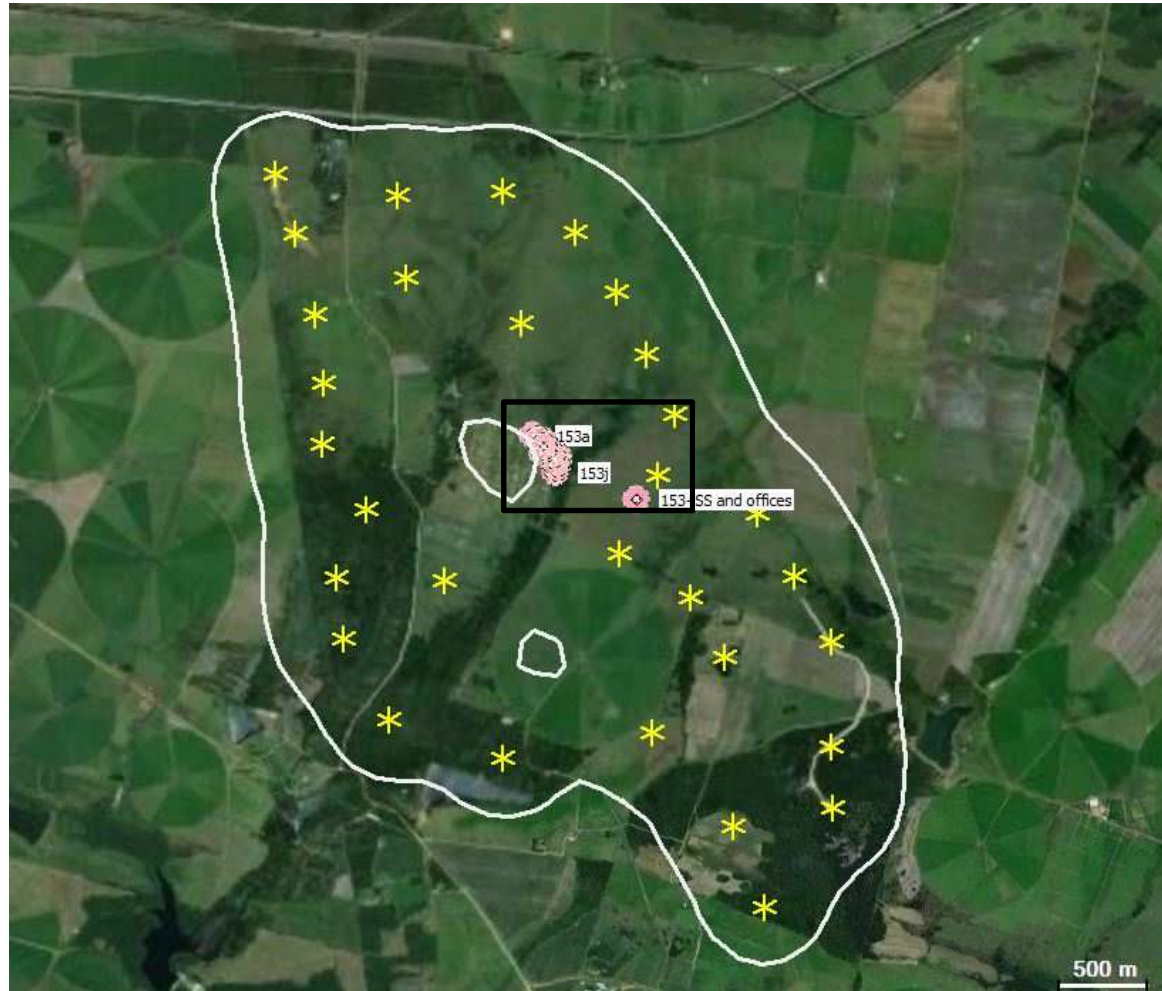
Figure 15: Noise contour map (45dB(A)) - Receptors with exceedance- Detail Tsitsikamma Community Wind Farm
