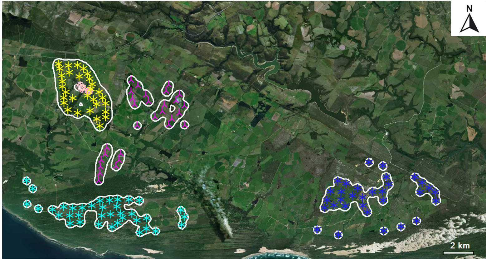
Figure 8: Noise contour map (45dB(A)) – Impact Assessment scenario (White line: 45dB(A) contour lines, pink circles receptor with exceedance of 45dB(A) limit, Magenta: Impofu West Wind Farm under study, blue: existing KWF, light blue: existing Gibson Bay Wind Farm, yellow: existing TCWF)
