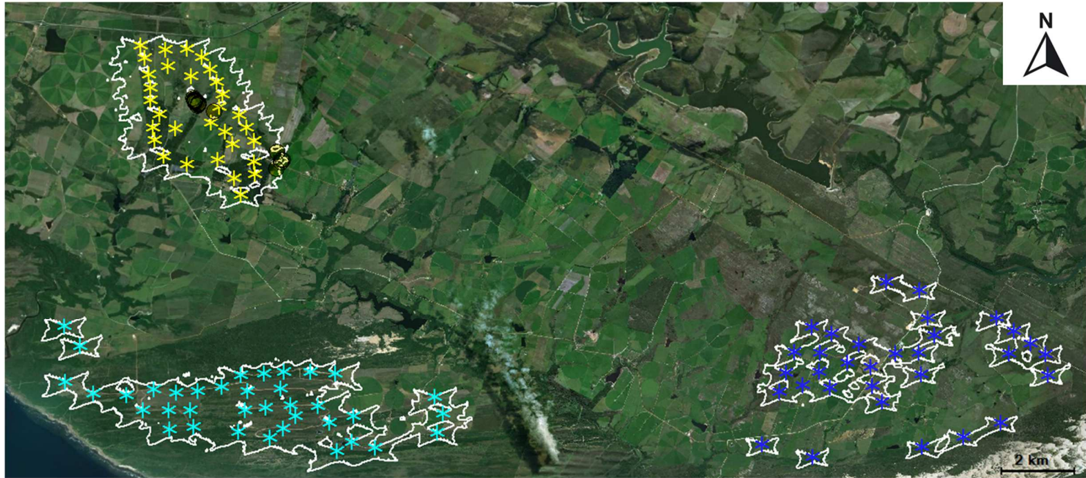
Figure 11: Shadow contour map (30h)- Baseline scenario (White line: 30h/yr contour lines, black circles: receptors with exceedance of limit, blue: existing KWF, light blue: existing Gibson Bay Wind Farm, yellow: existing TCWF)
