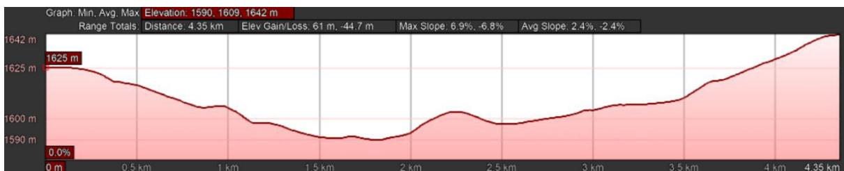
FIGURE 10-6: ELEVATION PROFILE OF PROPOSED PIPELINE
