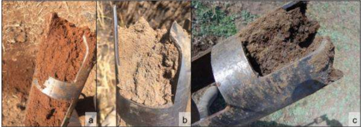
Figure 10-12: Characteristic soil forms identified on site showing: a) terrestrial soil, Hutton form; b) bleached E-horizon wetland soils found in the hillslope seeps, typical of Kroonstad form; and c) soils with mottling present and higher organic carbon content, typical of the valley bottom wetlands with Arcadia soil form
