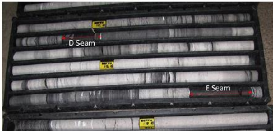
Figure 11: Borehole core photos showing D&E Seam in the project area.
