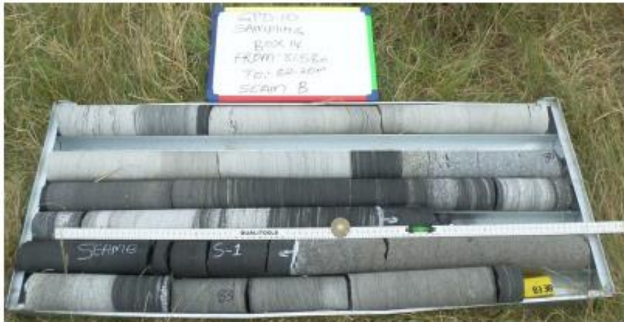
Figure 16: Borehole core photos showing B-Seam in the project area.
