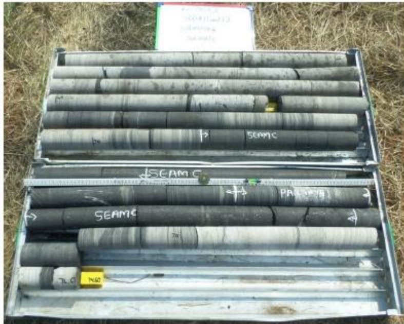
Figure 12: Borehole core photos showing C-Seam in the project area.
