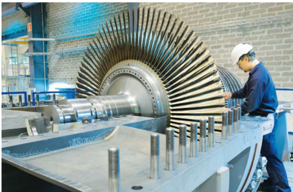
Figure 2.3: The steam turbine rotor, primary component of a steam turbine (Source: Siemens AG)
