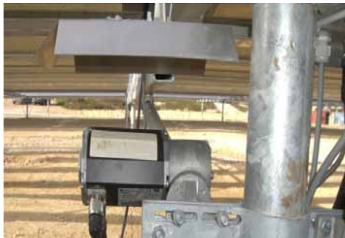
Figure 2.8: Tracking motor (Source: Novatec)
