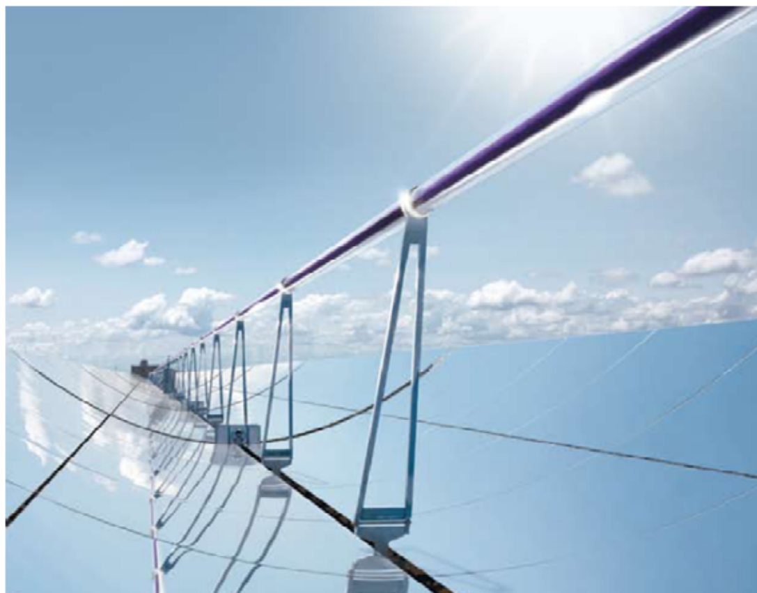
Figure 2.1: The top photograph illustrates the pipes conveying the heat transfer fluid and the bottom photograph illustrates the parabolic troughs together with the receiver tube (Source: Siemens AG)
