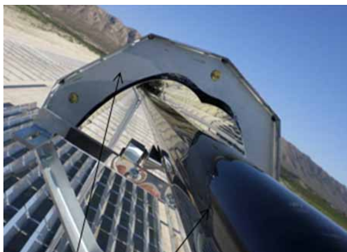
Figure 2.7: Receiver and Secondary Reflector Primary reflector (Source: Novatec)
