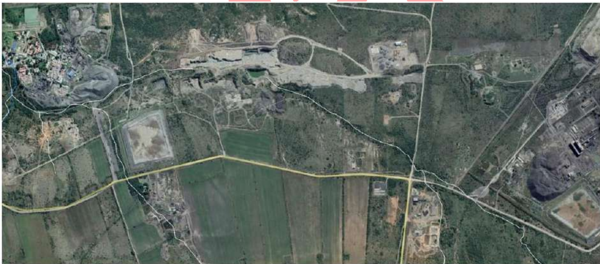
Figure 20: All aspects affecting the reach of the Southern tributary of the Marelwana River. Note the development of the Elandskraal Chromium mine directly through the watercourse (Google Earth, March 2020)
