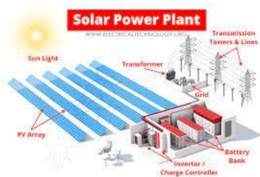
Figure 2.4: Overview of Solar PV Power Plant
