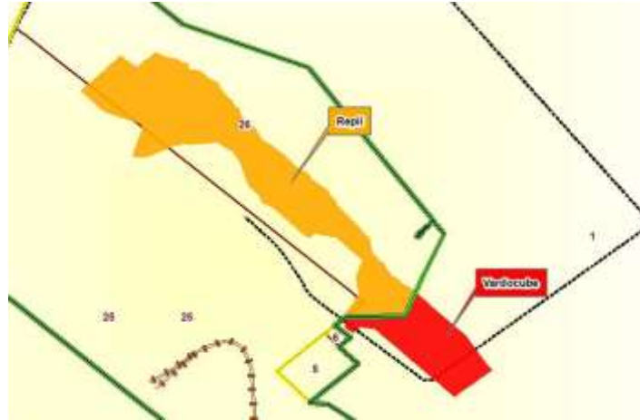
Figure 6. Plan showing the relative position of the Vardocube extensions to the Repli Section of the proposed underground mining area. Area 5 is the Eskom Yard and 6 is a steel tower.
