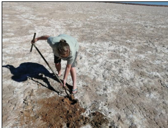
Figure 10: Photograph of infield soil analysis via hand-held Dutch soil auger on Grootwitpan
