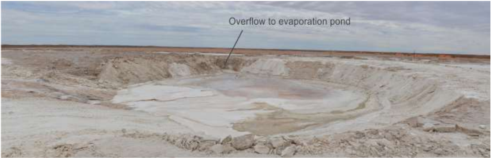
Photo 9: The water removed by the cyclone is fed to this pond which evaporates to yield very fine salt in small quantities
