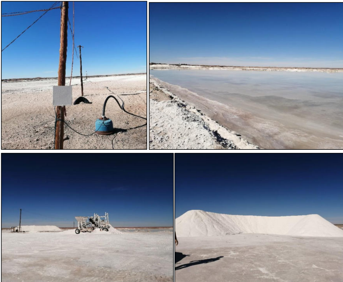
Figure 13: Top left: A pump to transport the brine from below the pan surface to ponds above. Top right: An evaporation pond on the pan. Bottom left: a salt sorting/rinsing area. Bottom right: A salt stockpile ready for loading and transport to Upington
