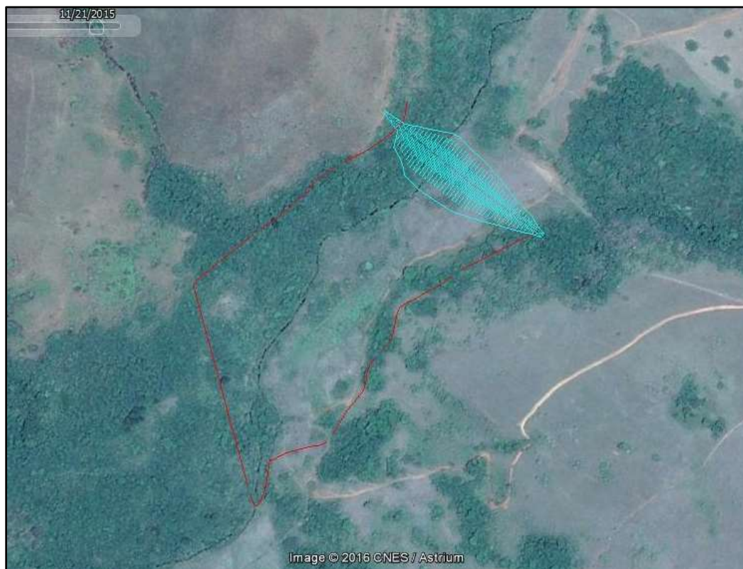
Figure 6.2.3. Preferred dam wall site and footprint area- full supply level (FSL).
