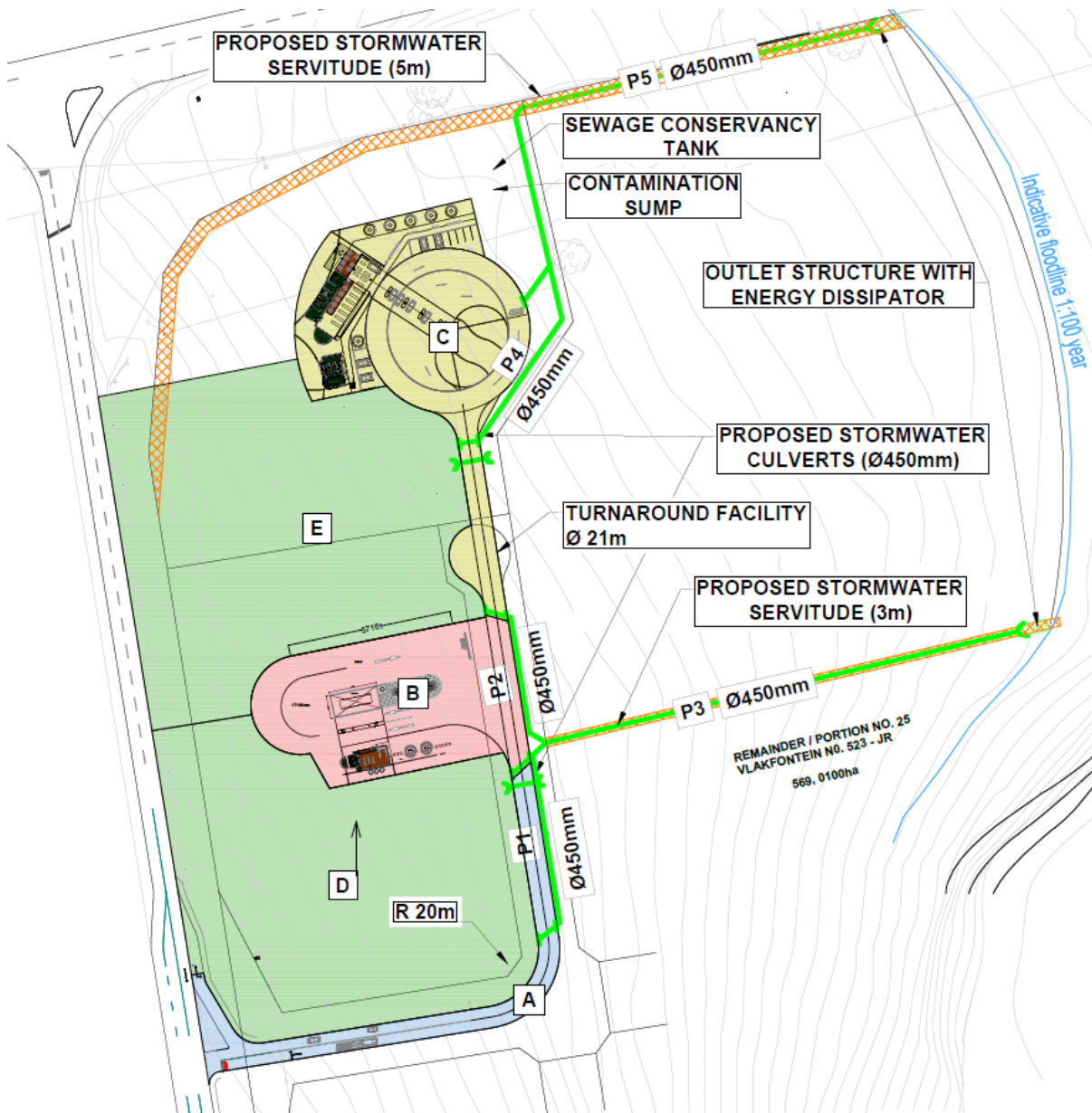
Figure 3: Storm water layout
