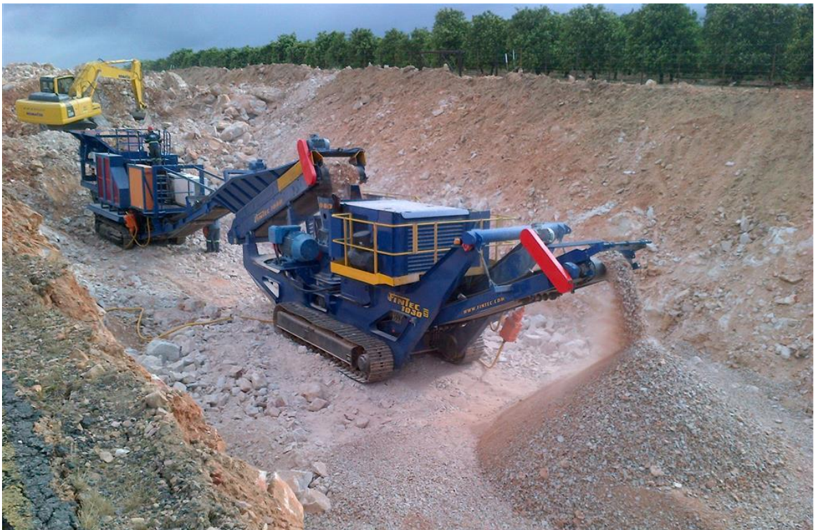
Photo 3: Typical mobile tracked in-pit crusher
