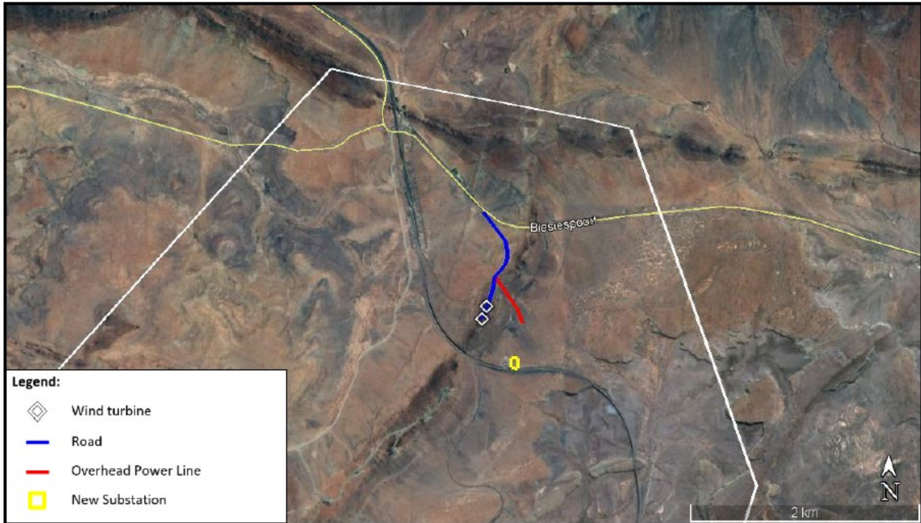
Figure 3: Layout for the proposed road, OHPL and two upgraded wind turbines, showing the Noblesfontein Site's northern boundary, completed turbines to the southwest, and the position of the proposed second substation adjacent to the existing substation.
