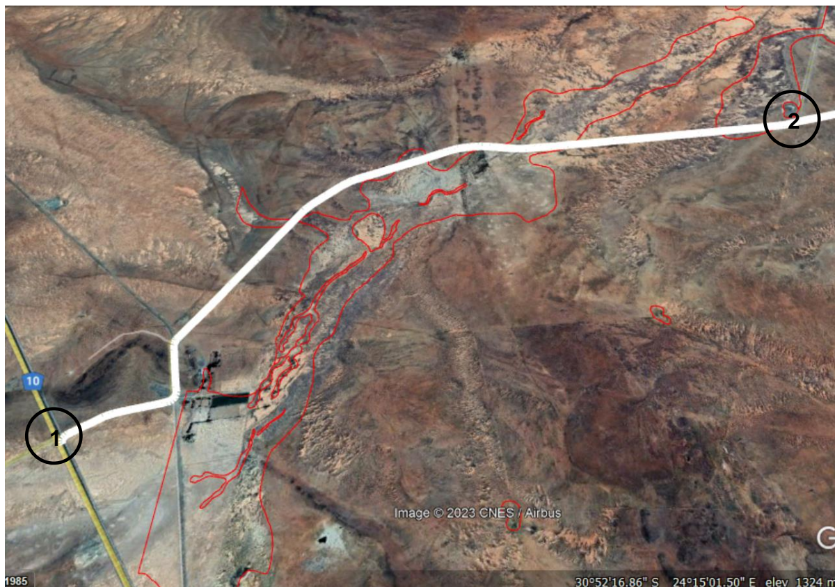
Figure 2. Section of existing public 'Burgerville' District Road (2448) from its intersection with the N10 (1) to its intersection with the existing private road (farm track) at the boundary of Farm Riet Fountain 39C (2). Red lines indicate flood plain soils (possible watercourses).
