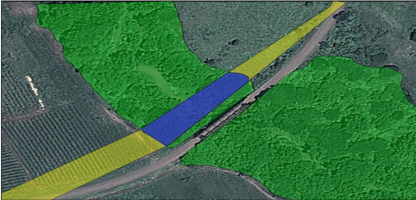
Fig: 1 Preliminary sensitivity map for the proposed replacement of the Nseleni River Bridge at (11.3 km) on the P425 highlighting sensitive habitats along the proposed alignment. The Yellow area indicates transformed habitats of the proposed re-aligned P425 (Low Sensitivity). The Blue area indicates the proposed new Nseleni bridge alignment (High Sensitivity) and the Green area indicates the riparian zone of the reach of the Nseleni River (High sensitivity).
