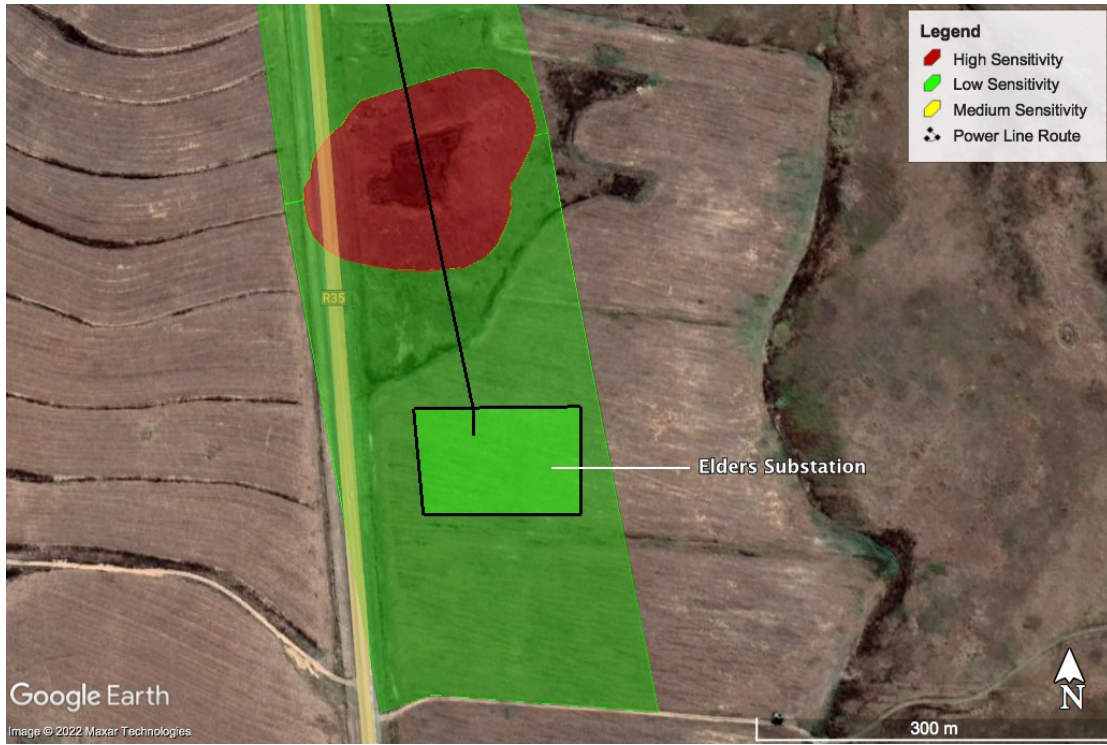
Figure 9: Sensitivity Map: Elders Substation
