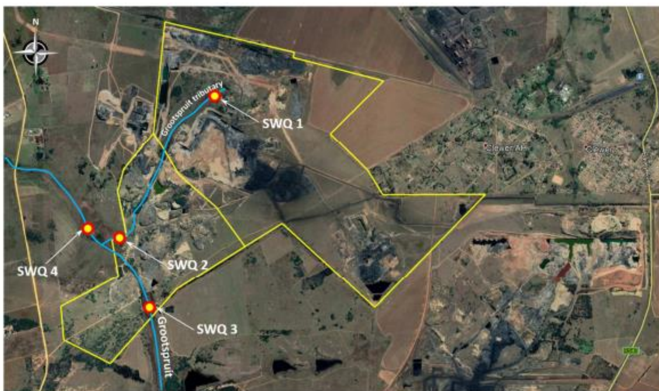
Figure 4: Minimum recommended surface water monitoring locations
