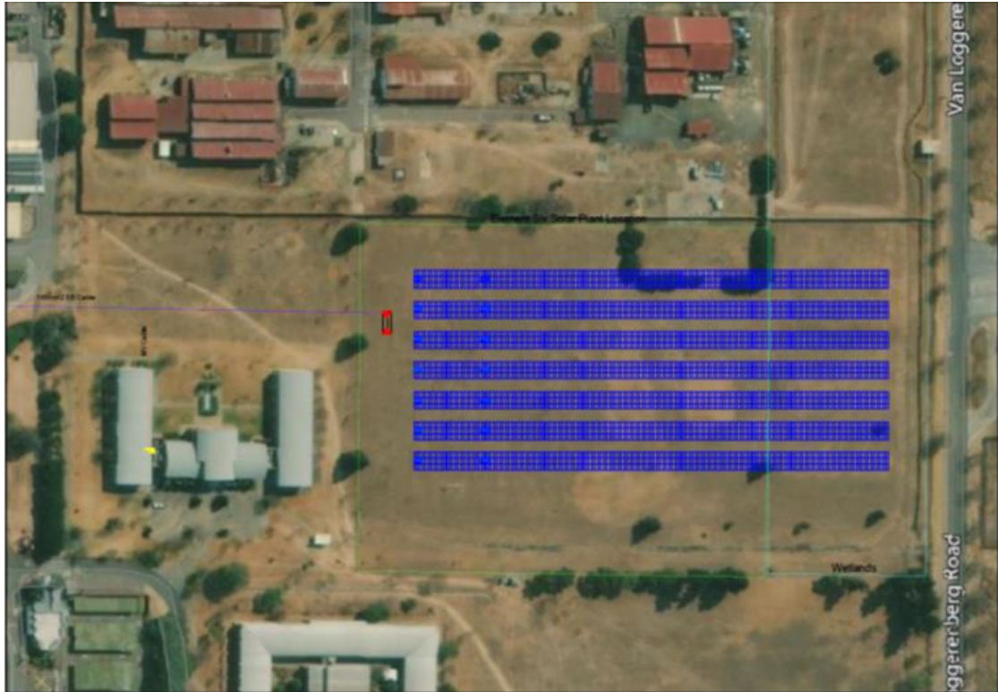
Figure 1. Solar PV facility presented relative to the Element Six buildings and alignment of 6.6kV sub-surface cable (purple line) leading from the RMU (red polygon).
