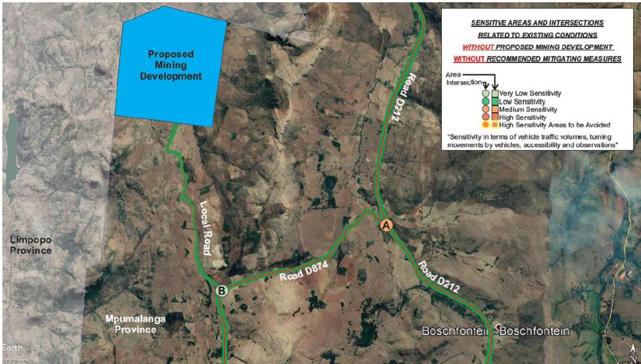
Figure 17: Sensitive road section and intersections indicating existing sensitive areas and intersections without the proposed mining development (status quo)
