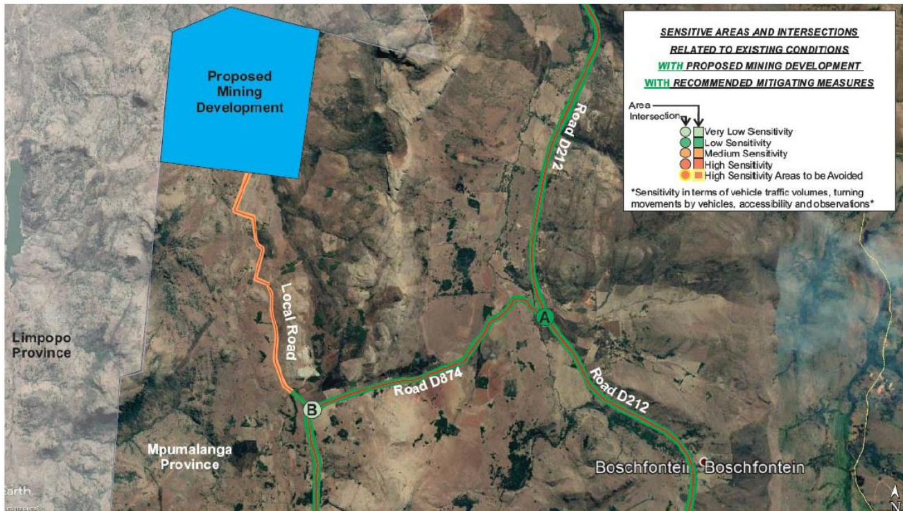
Figure 20: Sensitive road sections and intersections indicating anticipated sensitive area and intersections with the proposed mining development with mitigation measures
