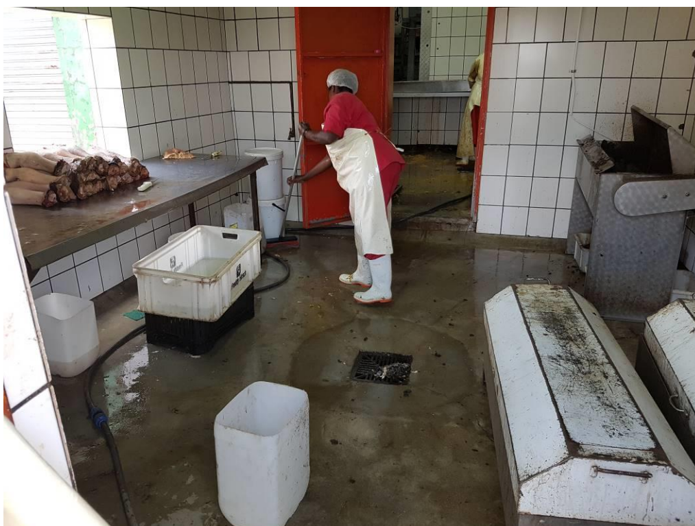
Photograph 2: Example of Dressing Area. Waste water contains some blood, fat and off-cuts.
