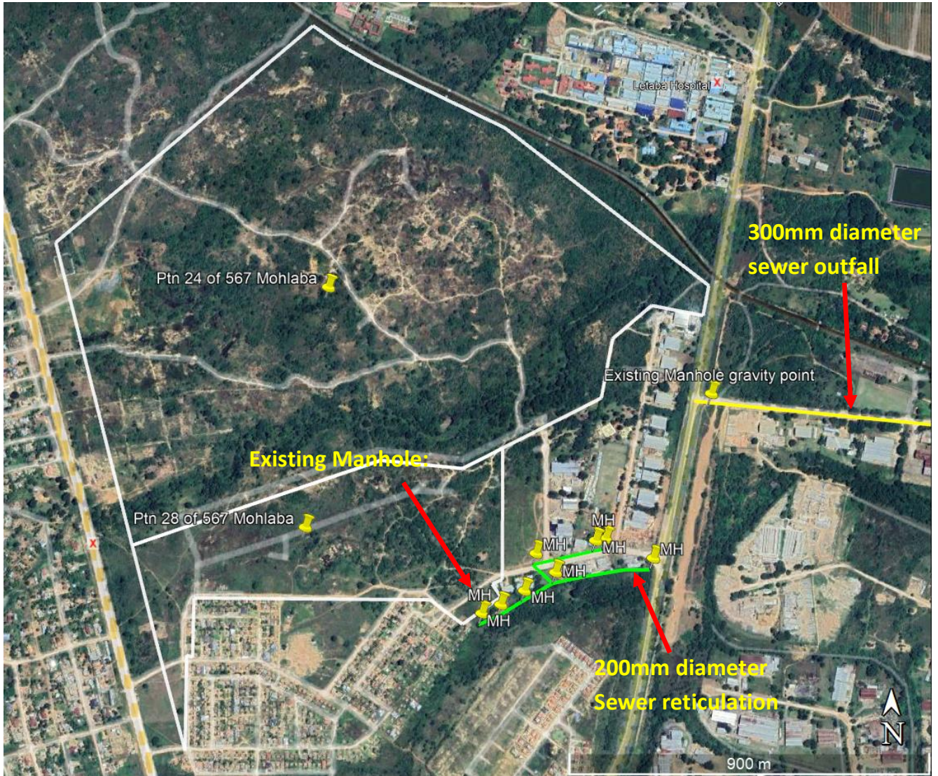
Figure 17 Existing sewer infrastructure
