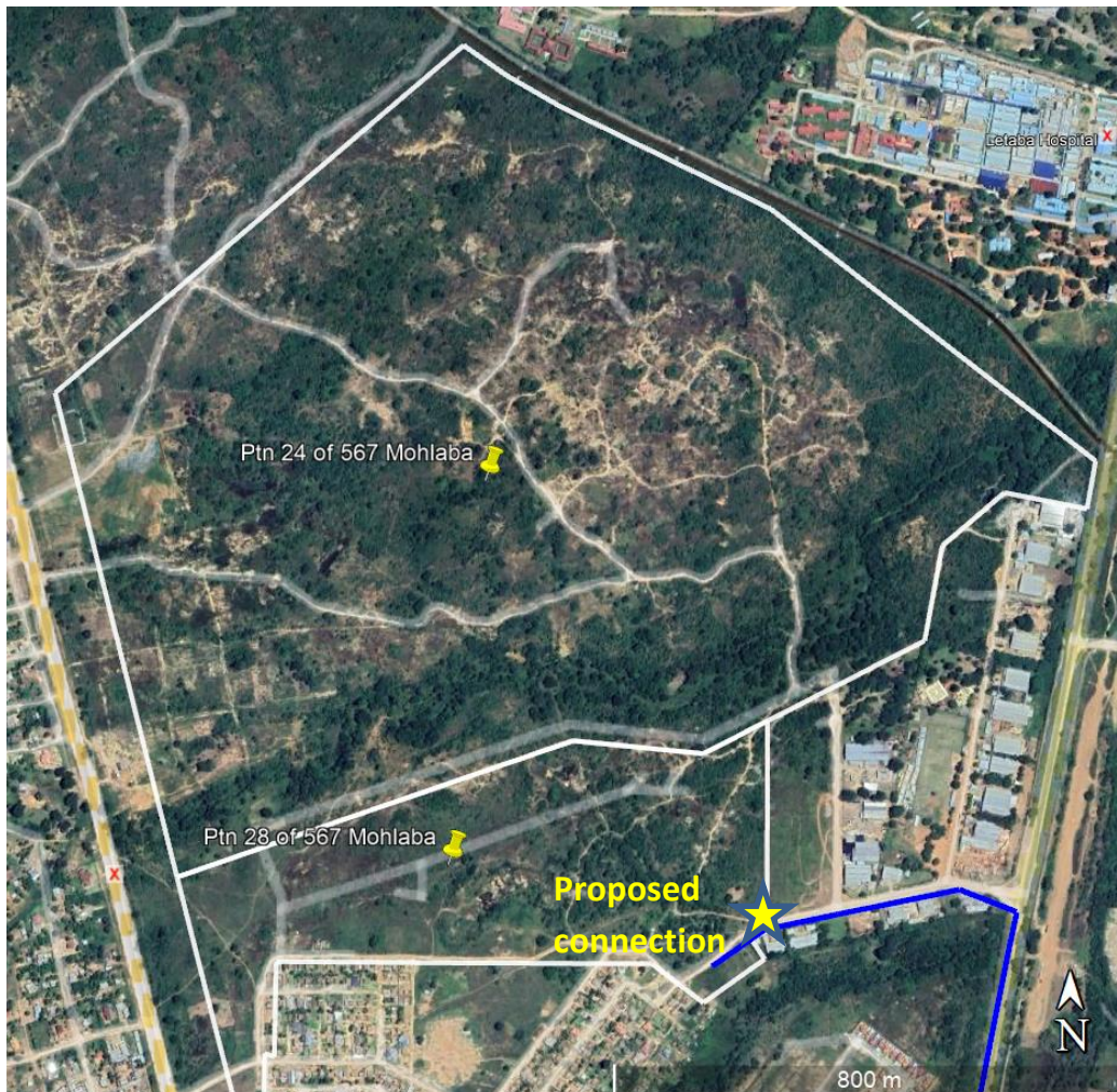
Figure 11 Proposed connection to the 200mm diameter bulkline (blue line)
