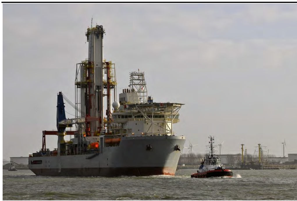
Figure 3.2 Example of a Drillship
