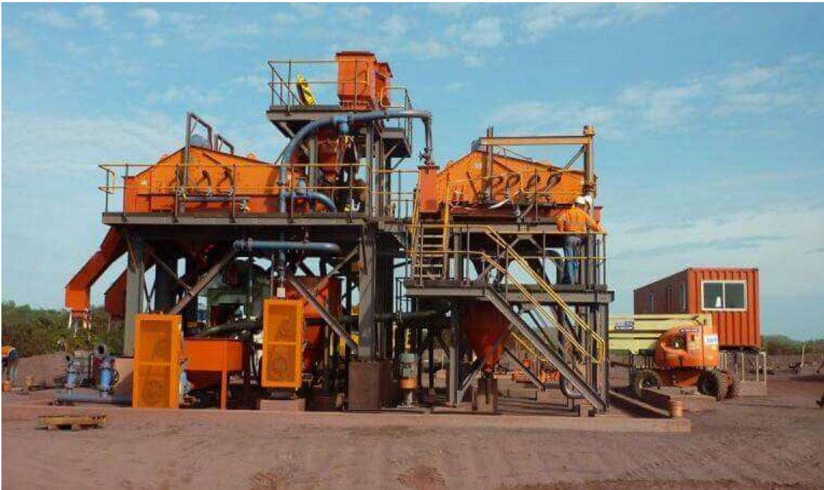
Figure 8: Dense Medium Separation
