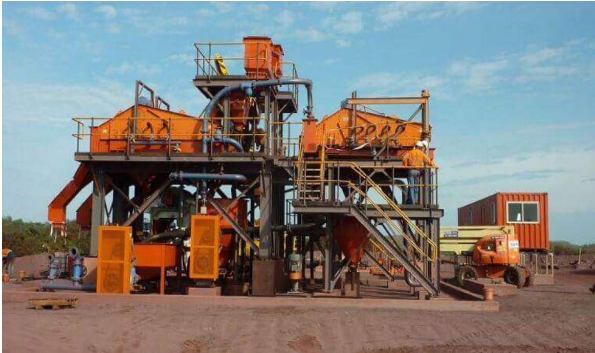
Figure 8: Dense Medium Separation
