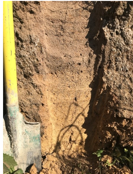
A vertical profile of soils within a transformed wetland area. This would have been an historical seasonal zone. Mottling is visible within the upper layers. The upper layer is also bleached (gleyed) as the iron pigment leaches. Desiccation of the soils due to channelling of the water within the wetland has led to soil destabilisation.
