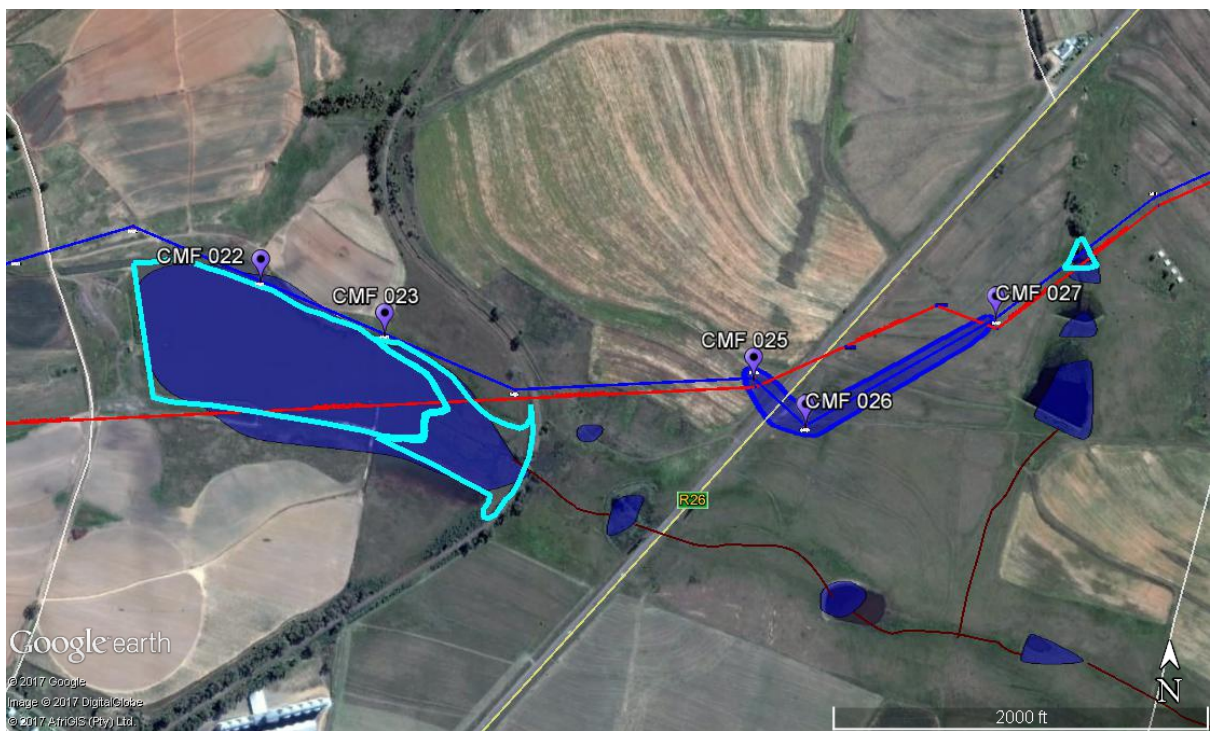
Figure 4 Poles 22, 23, 25, 26 and 27 are located inside, or within 32 m of an identified wetland / watercourse.
