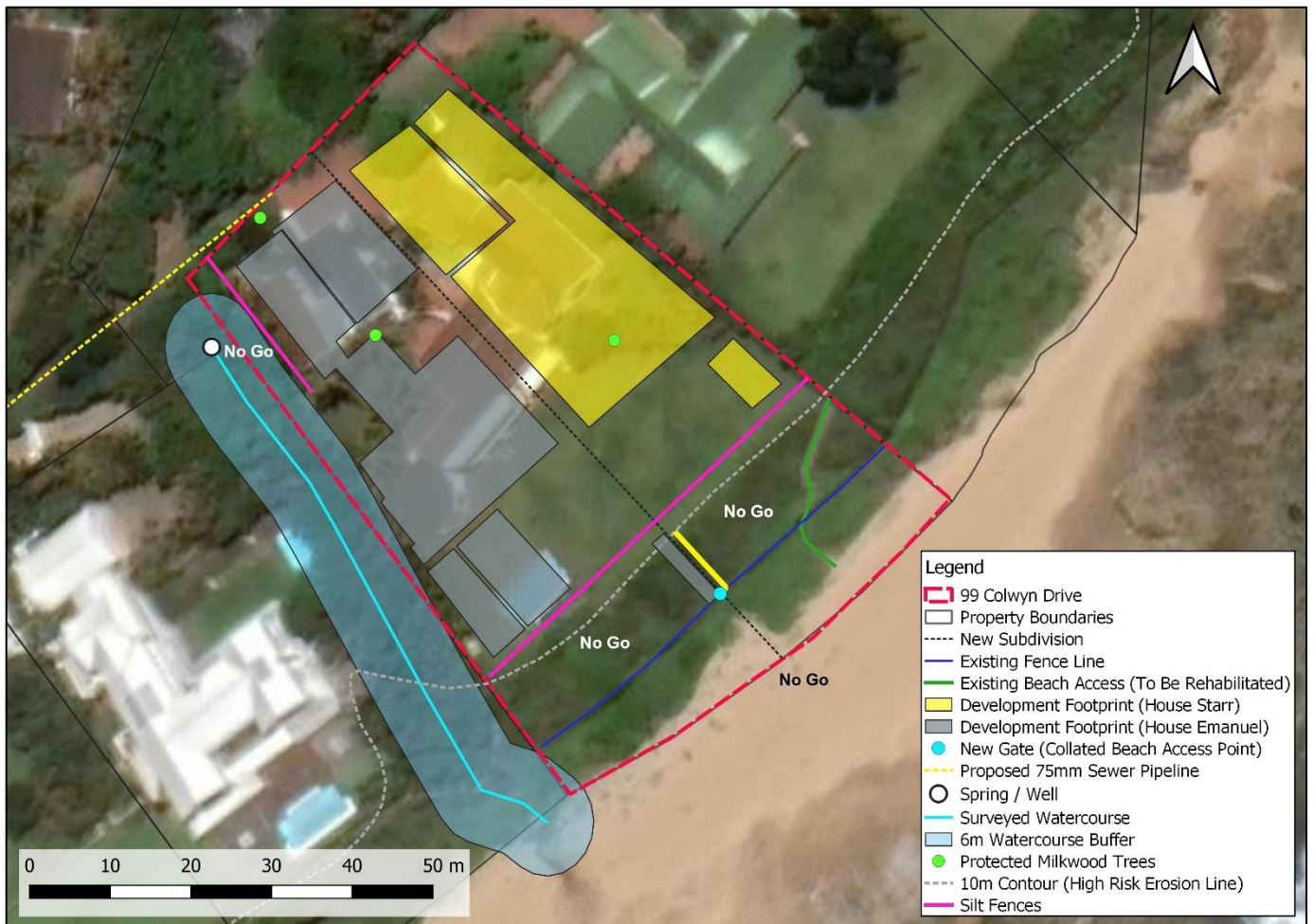
Figure 12: Location of House Emanuel (South) and House Starr (North) at 99 Colwyn Drive Showing Sensitive Environmental Areas to be Avoided During Construction.
