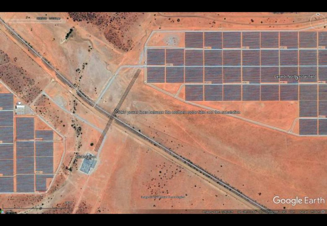
vi. To show PV arrays of up to 1km in length across the south solar field and up to 1,5km in length across the north solar field, and made up of approximately 100m sections
