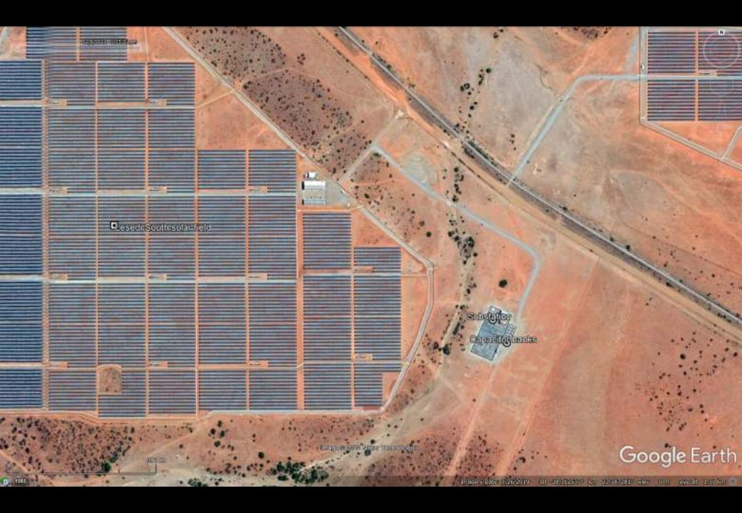
• iii. To indicate the location of the operations and maintenance facility, and to show this consists of an office and storage buildings, security, ablution facilities, parking, outdoor storage area and water treatment facility
