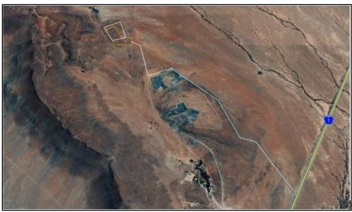
Figure 6: Satellite view showing the access road (white dashed line) to the proposed mining area site alternative 1(orange polygon) as well as site alternative 2(white polygon).
