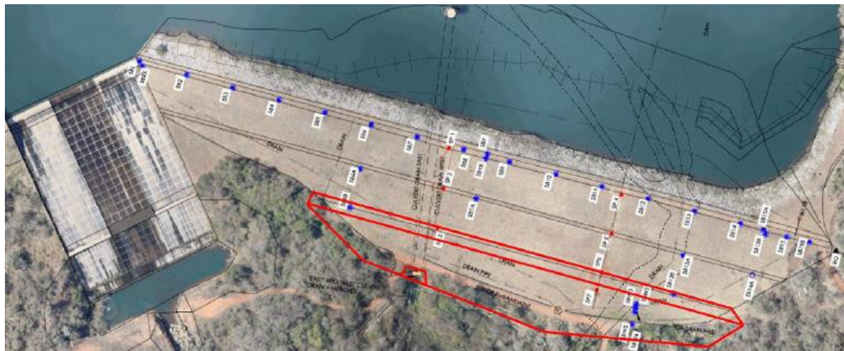
Figure 23. Ngodwana Dam wall with red area indicating the extent of the fill required on the main embankment to provide the necessary slope stability.
