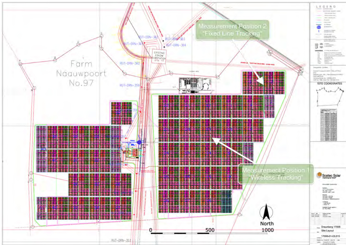
Figure 1: Diagram of plant layout showing measurement location at inverters 22 and 23.
