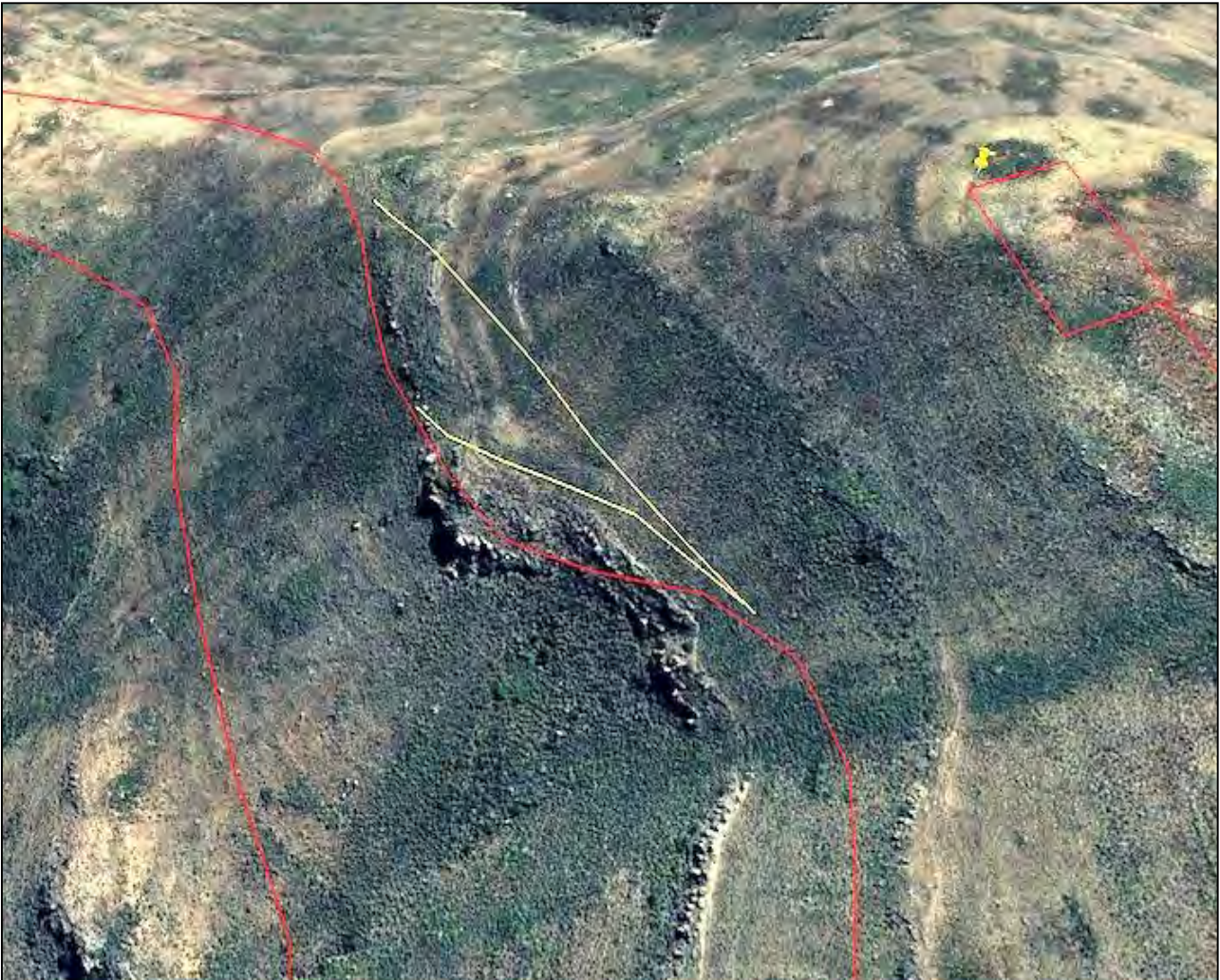
Figure 38: Proposed shift in position of internal access road between Turbines 28 and 29. (Road & crane pad boundary = red line, proposed re-alignment = yellow lines)
