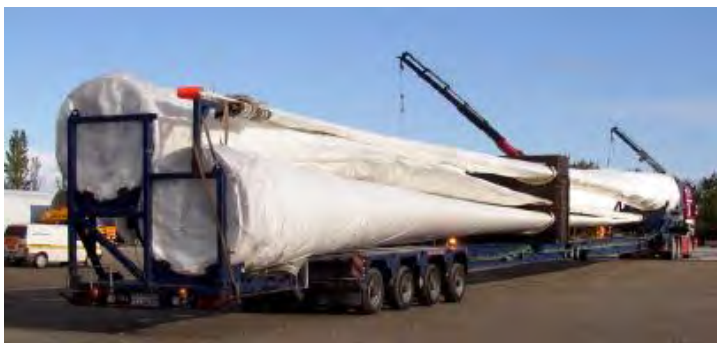
Figure 2: Example: 3 x 45m Blades on extendible trailers
