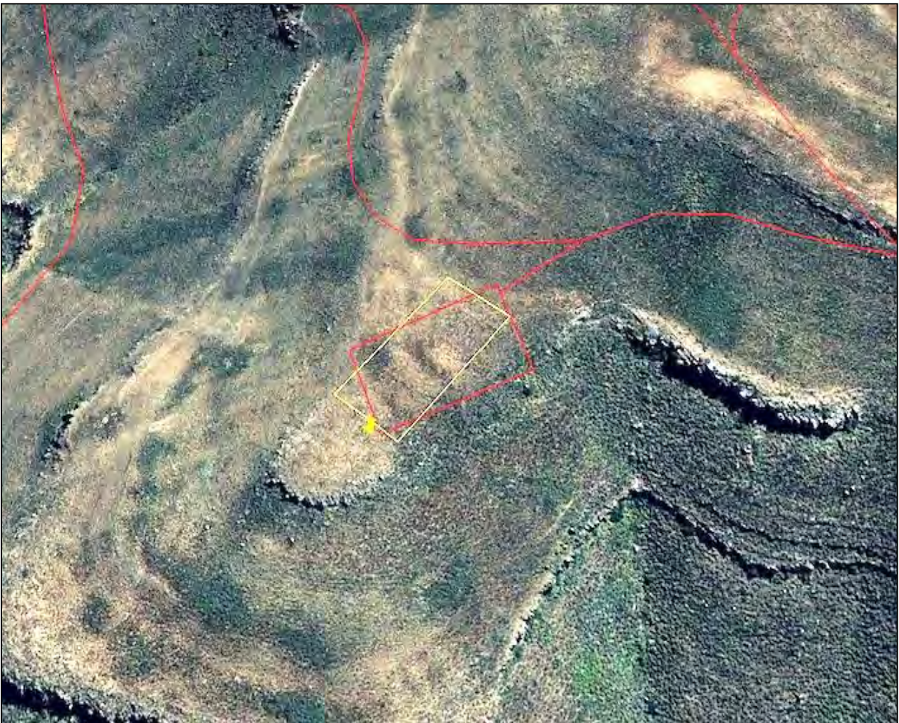
Figure 36: Proposed shift in position of crane pad at Turbines 29. (Road & crane pad boundary = red line, proposed re-alignment = yellow lines)
