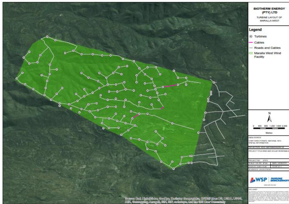
Maralla West Initial Turbine Layout (125 Turbines – 250 MW)
